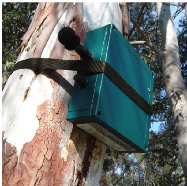
*The Song Meter SM2+ series from Wildlife Acoustics are compact and affordable digital audio/ ultrasonic recorders specifically designed for the automated recording of wildlife vocalizations. They are robust and weatherproof, suited to long term and unattended deployment in harsh outdoor environments.*
