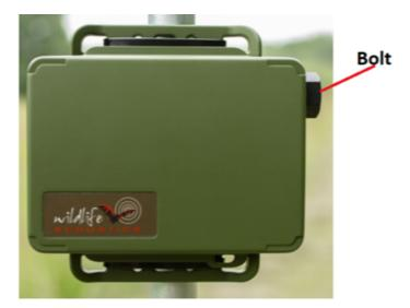
The first issue can affect both Song Meter Mini and Mini Bat recorders. The removable black plastic bolt, located at the top right corner of the recorder where the optional acoustic microphone can be added, has, in some cases, not been tightened to the proper specification during manufacturing. Note that this issue does **not** affect installed microphones (either from the factory or user installed).
