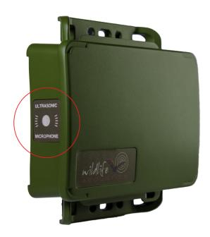
The second issue only affects Song Meter Mini Bat The label that covers the ultrasonic microphone on the left side of the recorder may not have been applied securely during manufacturing.
