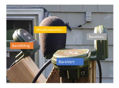
We found that orienting the SMM-U2 so the sensor is aimed horizontally, so that water cannot pool on top of the mic, will improve wet-weather recording when compared to orienting the SMM-U2 so the sensor is facing the sky. However, windblown rain or condensation can still cause water to collect in the mesh, resulting in attenuation.
