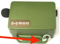
5) Place the cable straight toward the right so the cable goes through the right-side notch in the AA battery tray. (If the cable isn't in the notch, it will get pinched and the lid cannot be fully closed).
