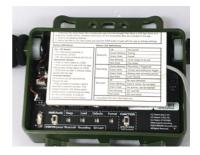
8) Insert batteries in pairs as needed. When closing the lid, be careful to avoid pinching the cable. Seat the extra cable length under the metal bracket and close the lid. It should snap on both sides to create a weatherproof seal. See the Mini user guide for more information.
