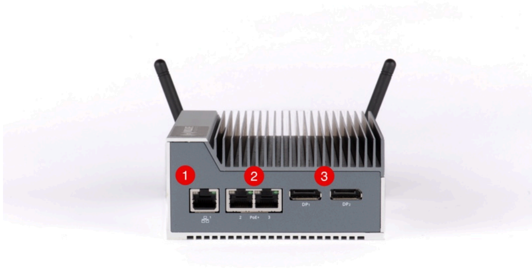
Figure 1. SMART Controller Connectivity: Ethernet and DisplayPort
