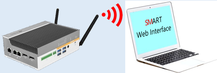
SMART Controller is WIFI HotSpot (Default configuration)
