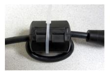
1. As near to the microphone as possible, loop the cable through and snap the ferrite shut. A zip tie is included for further securing the ferrite.
